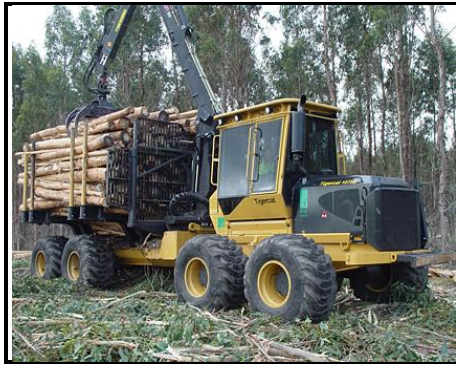
Forwarder machine used when extracting logs infield to the depot or landing
